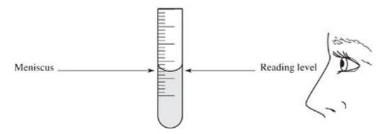
Use a *graduated cylinder* to measure liquid; and use the *meniscus* (bottom of the curve) at eye level to take your measurement.
