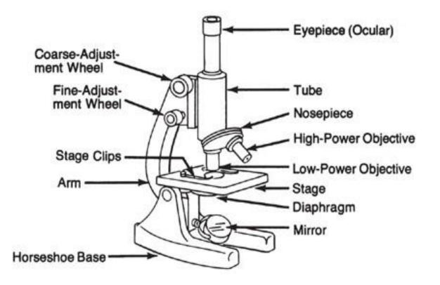
To determine the **total magnification**, multiply the magnification of the ocular lens or eyepiece by the magnification of the objective lens.
