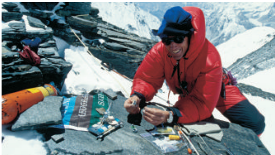
■ Figure 1-14 A series of expeditions succeeded in placing a GPS receiver on top of Mount Everest. This improved the accuracy of the altitude measurement: Everest's peak is 8850 m, not 8848 m, above sea level.
