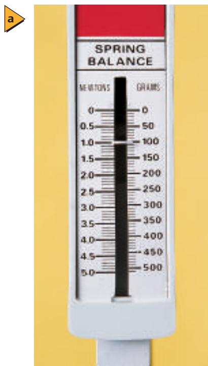
■ Figure 1-13 By positioning the scale head on (a) , your results will be more accurate than if you read your measurements at an angle (b) . How far did parallax shift the measurement in b?
