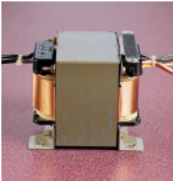
Figure 25-14 If the input voltage is connected to the coils on the left, where there is a larger number of turns, the transformer functions as a step-down transformer. If the input voltage is connected at the right, the transformer functions as a step-up transformer.
